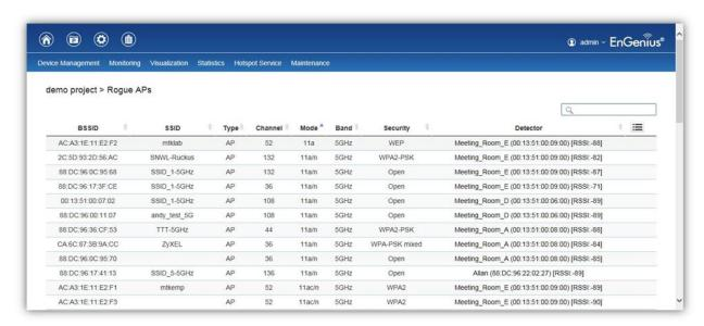
Rogue Access Points refer to those unauthorized and often unmanaged APs attached to an existing wired network which could bring harm to the network or may be used to deliberately gain access to confidential company information. With *Background Scanning* enabled, the Rogue AP Detection feature can be used to periodically scan 2.4 GHz and 5 GHz frequency bands to identify rogue wireless Access Points not managed by the ezMaster.
