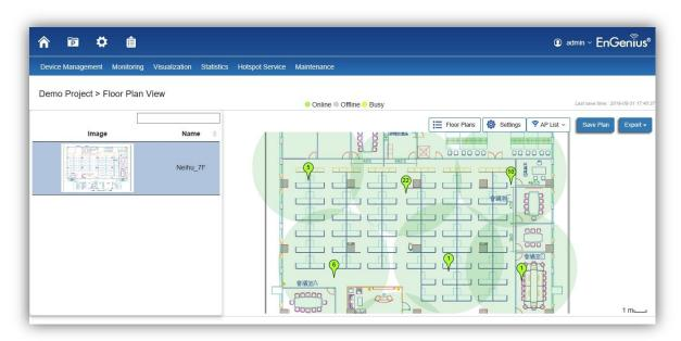
After importing your floor plan image, you can distribute markers that represent the APs to the correct locations by clicking on **AP List** and dragging each marker icon to its correct location on the floor plan. Also, Wireless Coverage Display can be toggled on to indicate the coverage range of each AP, assisting IT managers to easily and accurately plan and deploy wireless networks in any indoor environment. Click on **Save Plan** when you're done to save settings.
