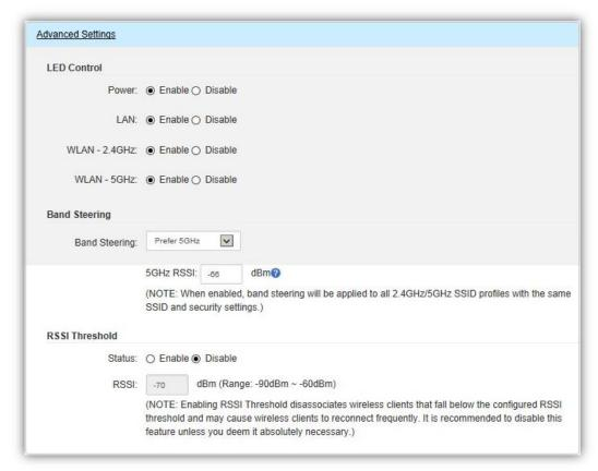
**LED Control**: In some environments, the blinking LEDs on APs are not welcomed. This option allows you to enable or disable the devices LED indicators. Note that only indoor models support this feature.
