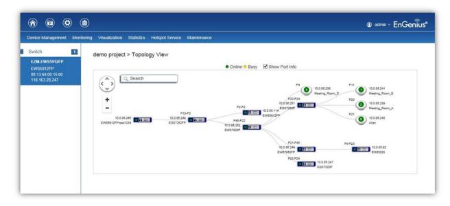
If you have an EWS Switch deployed in your network, you will be able to see a visual view of the topology of all supported devices in the network. The Topology View feature will automatically maps your network deployment and displays the device relationships across your network infrastructure. An essential feature for troubleshooting network issues that would otherwise require manual mapping, overlay monitoring software, or manually keeping track of MAC address tables.
