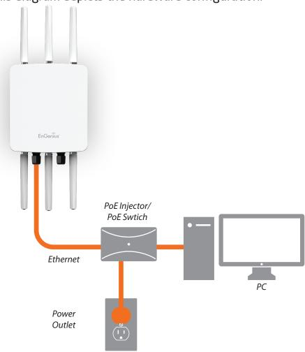
**Note:** The Access Point supports both IEEE 802.3at PoE (Power over Ethernet) or the included power injector. You may use either one as the power source. **Do NOT use both at the same time.**
