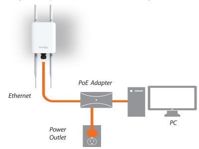
**Note:** The AP/Bridge should ONLY be powered via Ethernet cable connected to the included PoE Adapter.
