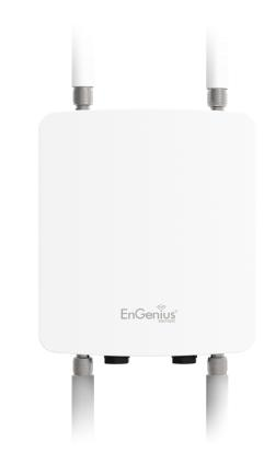
to a business network. The ENH710EXT supports the 2.4 GHz frequency band under 802.11 b/g/n mode while at the same time providing the 5 GHz band for communicating to and from other 5 GHz capable computers, tablets or smart phones or transferring files. Several ENH710EXTs can be deployed in a campus setting using the 5 GHz band as
