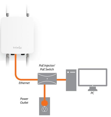
Note: The Access Point supports both IEEE 802.3at PoE (Power over Ethernet) or the included power injector. You may use either one as the power source. Do NOT use both at the same time.
